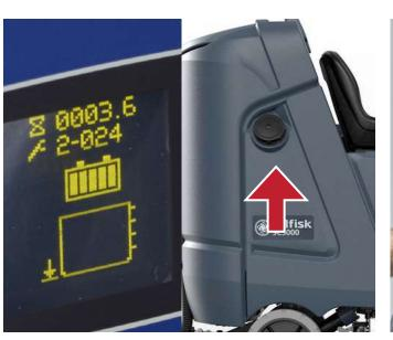
Fill the tank with a clean water. The clean water temperature must not exceed 40 °C. Make sure the solution valve under the machine is open.
