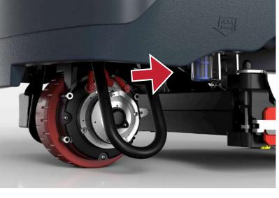
16. Clean the filter:A) Close the solution valve under the machine.B) Remove the transparent cover and the gasket, then remove and clean with fresh water the filter inside. C) Reassemble the filter.
