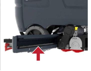
13. Slide out, check, empty and clean the debris cage (cyl version)
