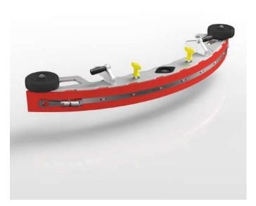
15. Untighten the yellow knobs, take the squeegee off and remove debris. Check and clean the squeegee blades.
