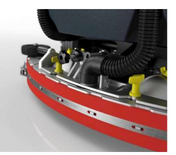
5. check the squeegee blades are not damaged and install the squeegee by turning the yellow knobs. Check the height of the squeegee by adjusting the castor wheels and the angle knob.
