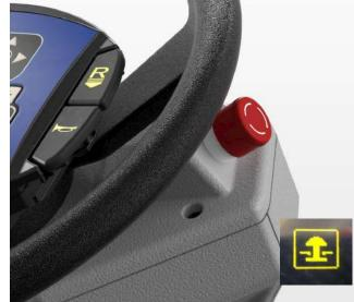
2. E-stop icon appears on display when E-stop switch is engaged. Twist Estop switch to enable machine function.
