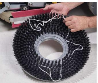
14. Turn the brushes counter clock wise and remove the brushes or pad holders. Rinse the brushes or pads in warm water and hang up to dry.
