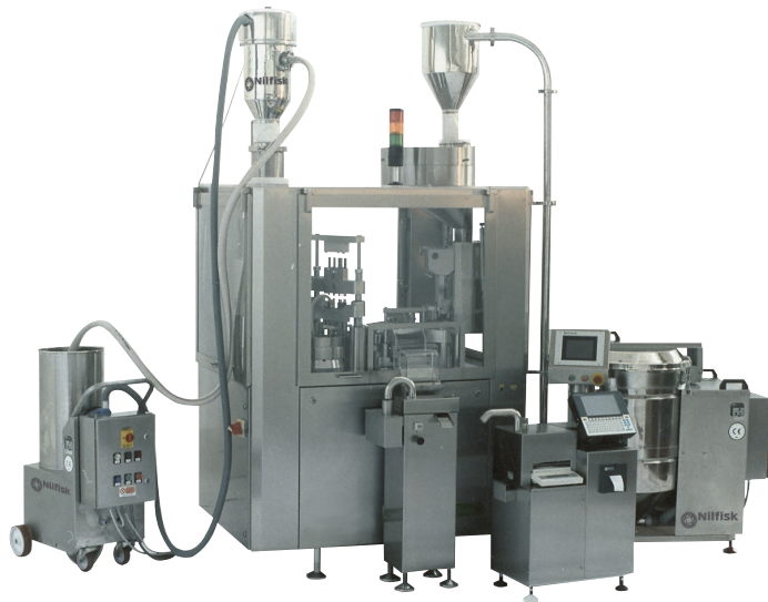
Pneumatic conveyor (left) and capsule pusher (right), in a pharmaceutical company.
