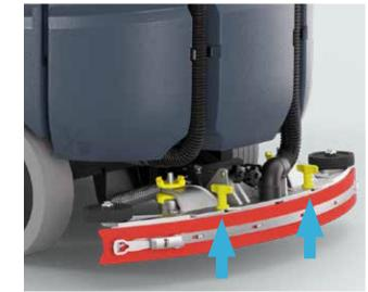
5. Check the squeegee blades are not damaged and install the squeegee by turning the yellow knobs. Check the height of the squeegee by adjusting the castor wheels and the angle knob.
