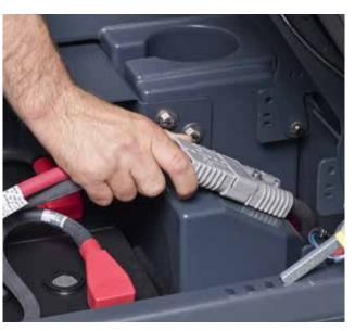
**3.** Check battery cables are well connected together.
