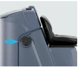
Fill the tank with clean water. The clean water temperature must not exceed 40 °C (104F).
