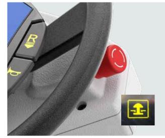
2. E-stop icon appears on display when E-stop switch is engaged. Twist E-stop switch until it pops out to enable machine function.
