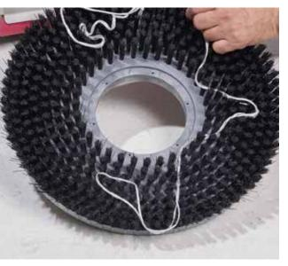
**3.** Turn brushes counter clockwise and check if there are external materials entangled and impeding efficient working order.
