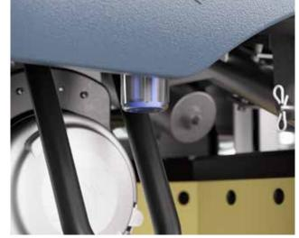
2. Verify solution is flowing to the deck. If not, verify solution tank is not empty and solution valve is open.
