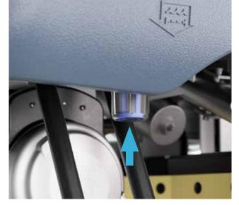
**3.** Check if the solution filter is cleaned.
