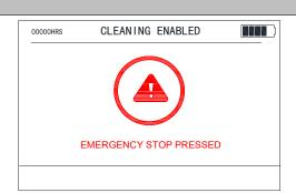
All functions are turned off. After releasing the emergency stop button, the machine needs to be restarted by pressing the Power button to restore normal operation.
