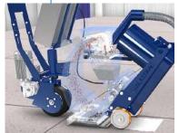
Connection to shot blasting machines for the collection of cement debris – process operation
