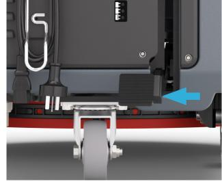
**2.** Lift the deck by pressing the pedal.
