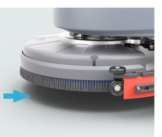
**3.** Place the brush or the pad-holder under the deck and lower the deck or the brush/padholder by pressing the pedal.
