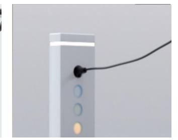
**18.** Daily: Charge the batteries: Connect the battery charger cable to the electrical socket. Light turns red when charging and green when the charging is complete.
