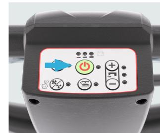
**4.** With the machine on, press one of the safety switches to engage the brush/pad-holder, then release it. If necessary, repeat the procedure until the brushes/pad-holder is engaged. The squeegee is raised and lowered with the deck.
