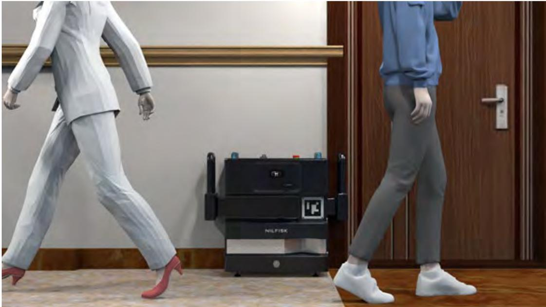
Docking Station should not be placed near doors, or area with high human traffic
