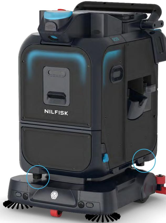
LIDAR use pulsed light waves to detect objects when the light waves are rebounded back. The object's distance is calculated based on the time it takes to rebound back.
