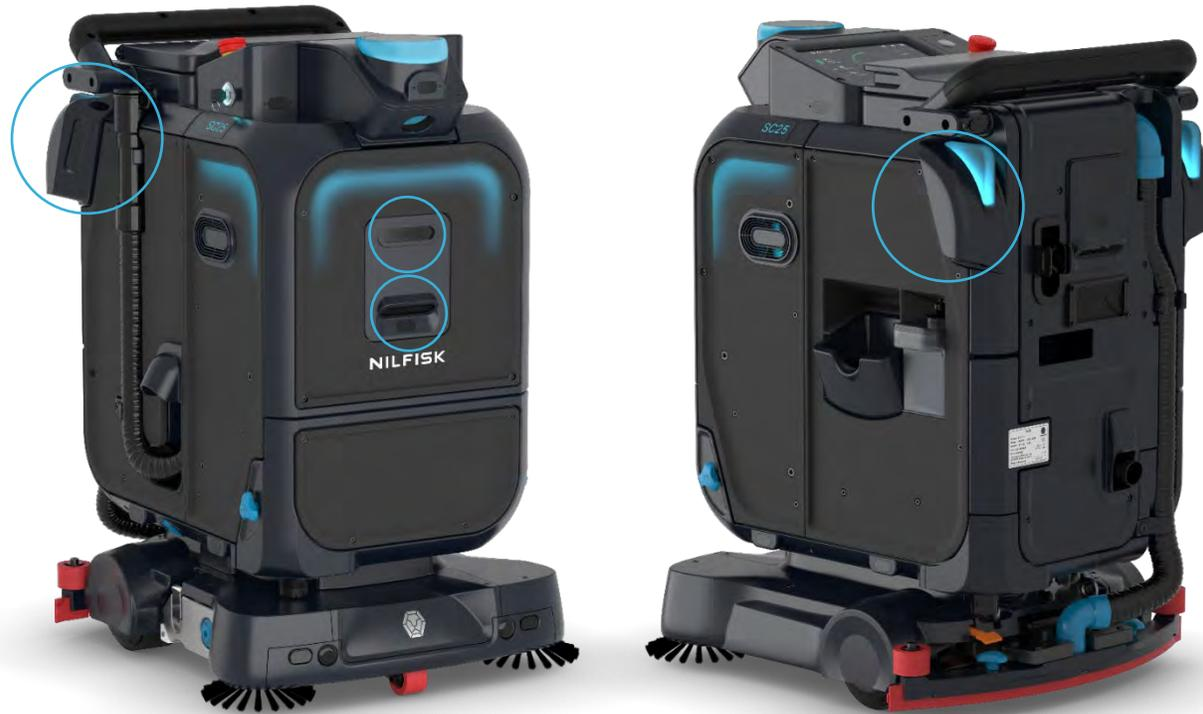
Uses IR projection to estimate depth of images. RGB image gives the robot a better understanding of the environment. The camera is able to detect and segregate objects.
