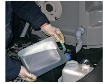
**4.** Fill the EcoFlex tank with a detergent suitable for the work to be performed (highly concentrated low foaming detergent).
