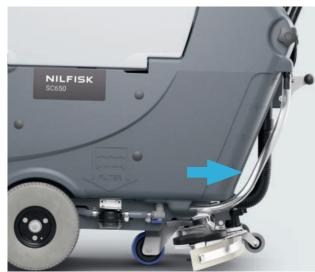
**3.** Check the solution level on the left side of the machine.
