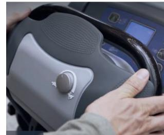
**10.** Push gently the drive paddle forward to start cleaning, control maximum speed with the speed dial, push the paddle backwards to go in reverse.
