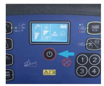
1. Turn on the machine and type in your default code 1, 2, 3, and 4 to verify there is enough battery power to complete the work. Charge batteries if required.
