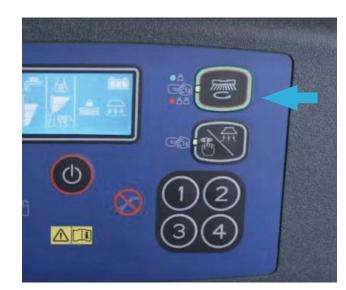
**6.** Lower the deck by pressing the Green button. To engage the brushes, slightly press the drive paddle and then release it.
