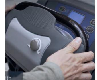
**3.** The machine does not move and the display shows: (WARNING ALARM E27) Machine is turned on with drive paddle pressed. Release the paddle and try again.
