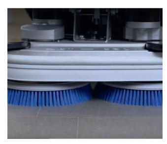
**5.** Place the brushes or the pad-holders under the deck. Use the appropriate brushes/ pads to clean the floor.
