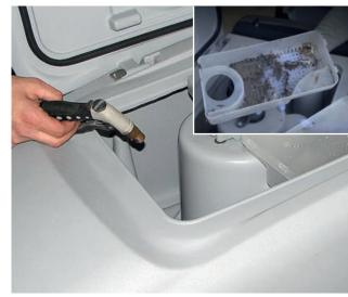
**13.** Wash with clean water the recovery tank and the vacuum grid. Remove, empty and clean the debris tray.
