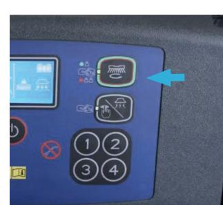
**4.** At machine start-up, the button LED flashes and the brushes do not work. Machine switched off without first raising the brush deck. Wait for the deck to raise before turning the brushes on again by pressing the button.
