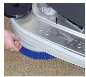
**1.** Check if the brushes are correctly installed and not worn out.
