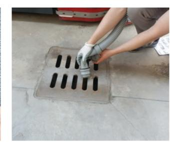
**13.** Empty the recovery tank with the hose. Then empty the solution tank with the transparent hose
