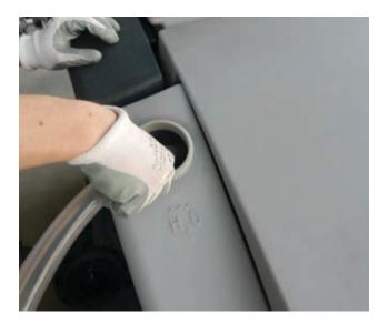
**6.** Fill in the DustGuard<sup>™</sup> water tank (if equipped)
