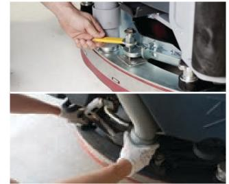
4. Install the squeegee and fasten it to its assembly then connect the vacuum hose to the squeegee. Make proper height and inclination adjustments
