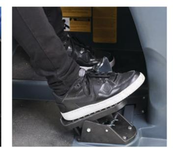
3. Drive pedal must be released during engine cranking
