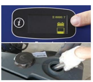
2. Check the fresh water level. In case, fill the tank with clean water. The clean water temperature must not exceed 40 °C
