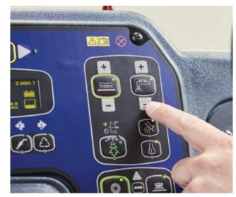
9. Adjust to the desired water flow
