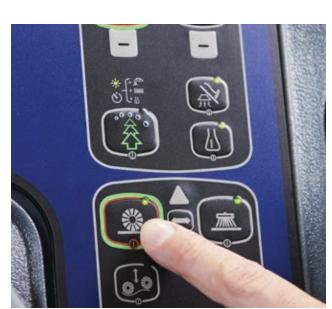
**4.** Adjust main broom pattern per operators manual to avoid overload condition. Inspect broom and drive for debris or adjust height if overload detected
