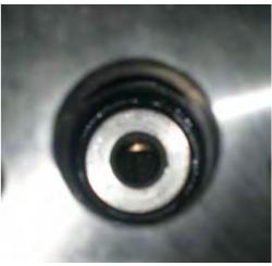
Use an O-ring picker tool to remove the O ring below the valve.
