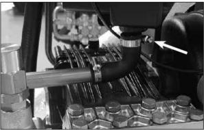
**Step 1:** Loosen the hose clip on the bent rubber angle at the outlet of the WBT and disconnect the two. If WBT is full, water will pour down over the pump.
