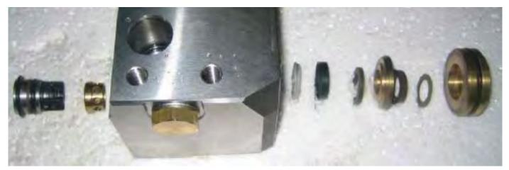
Disassembled view of pump head & manifold
