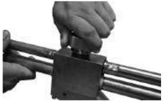
Using only your hand, unscrew the "Handi Change" cartridge nut located on the top of the gun block in a counter clockwise direction.
