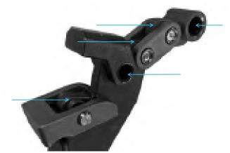
Lubricate the trigger in the indicated areas with a light oil.
