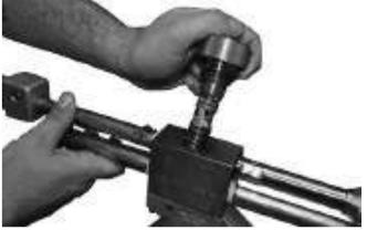
Pull up the cartridge assembly to remove it from its chamber inside the gun block.
