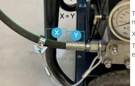
The high pressure hose connector safety device must be mounted correctly. See picture to the left.
