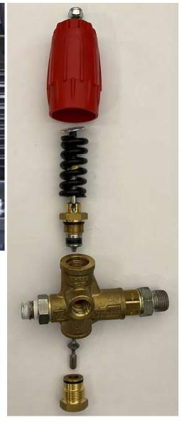
Every 500 working hours (approximately 12500 cycles of the system), check and lubricate the seals with water resistant grease.
