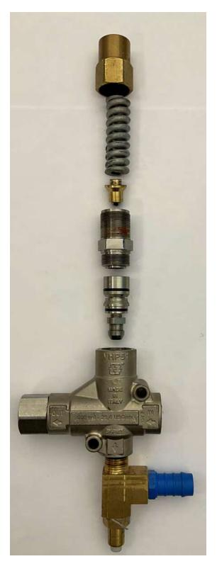
Every 500 working hours (approximately 12500 cycles of the system), check and lubricate the seals with water resistant grease.
