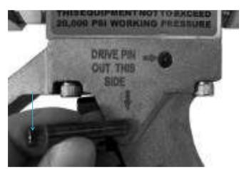
Insert and re-mount the trigger into the trigger gun from the oppo-site side of the trigger gun (Note: Verify you are inserting the pins from correct side by ensuring the text "Drive pin out this side" is present)
