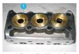
Insert the Pressure Ring (1) into the Pump Head, knock a few time with a mallet to compress the packing below
