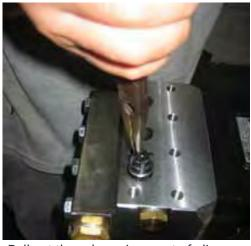
Pull out the valve using a set of pliers. Check the valves for damages, replace if needed.
