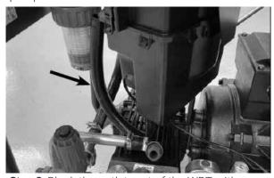
Step 3: Block the outlet port of the WBT with a short hose and turn hose upwards. Refill WBT so high that the level switch in the WBT will engage – enabling the VHPW to start up again.
