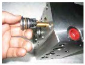
Push the valve out with a brass mandrel. Be careful not to scratch the inside of the pump head.
