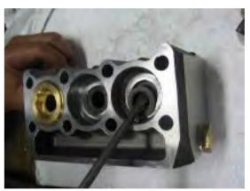
Use a screwdriver or pliers to fish out the packing.
