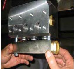
Loosen and remove the 10 mm bolts, except 2. Now remove the last 2 bolts and remove the manifold and pump head.
