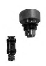
Using only your fingers, snap the cartridge assembly sideways out of the retaining groove at the lower end of the cartridge nut. Lubricate o-rings and seals. To assemble simply reverse the proces.
