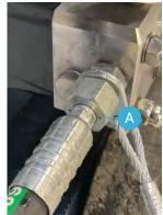
In the hose connection nut are drilled two pressure release holes. If pressure release of the high pressure hose is forgotten prior to disconnecting, these 2 holes will slowly release the pressure.
