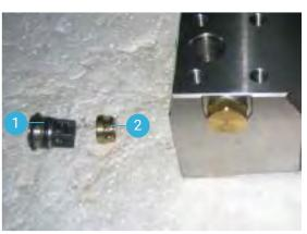
Check the valve (1) for damages, and replace if necessary.
