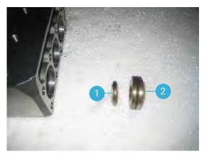
Push out the Pressure Ring (1) and the back ring (2) from the back with a brass rod. Be careful not to scratch the inside of the pump head.
