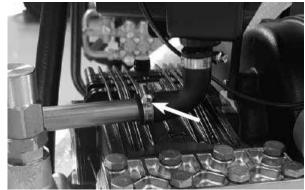
Step 2: Loosen the hose clip securing the bent rubber angle to the steel tube, turn the direction of the rubber angle to point outwards and tighten hose clip again.
