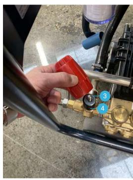
STEP 1 - Remove nut (1), handle (2), washer (3) and spring (4)
