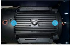
Motor for pump—grease points (1)
