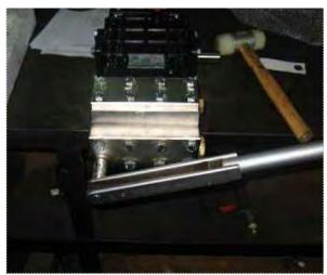
Teighten all bolts with the specified torque. Specifications below.
