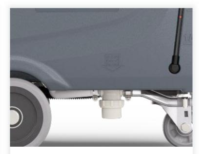
Solution filter enables operator to check and clean filter
